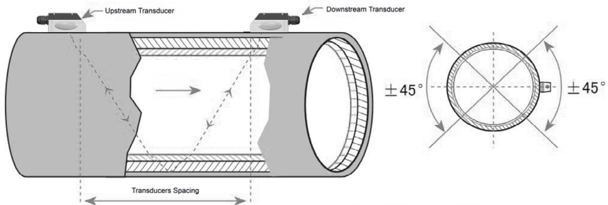
V-method installation is the most widely mode for daily measurement with pipe inner diameters ranging from 15 mm to 200 mm. It is also called reflective mode.
