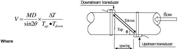
$\boldsymbol{\theta}$  is the include angle to the flow direction
