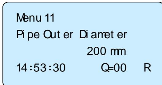
Visit Selection Type menus to check the related options. If need to modify it, press **Enter** first to enter the revised selection when the symbol “>” and a flashing cursor are displayed at the left end of the third line on the screen; or input numbers directly to select the option when the symbol “>” and a flashing cursor are displayed.
