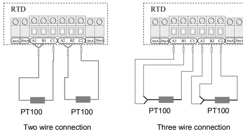
The two PT100 temperature sensors are installed on the inlet and return pipes and they will input temperature signals to the LRF-3000SW transmitter.
