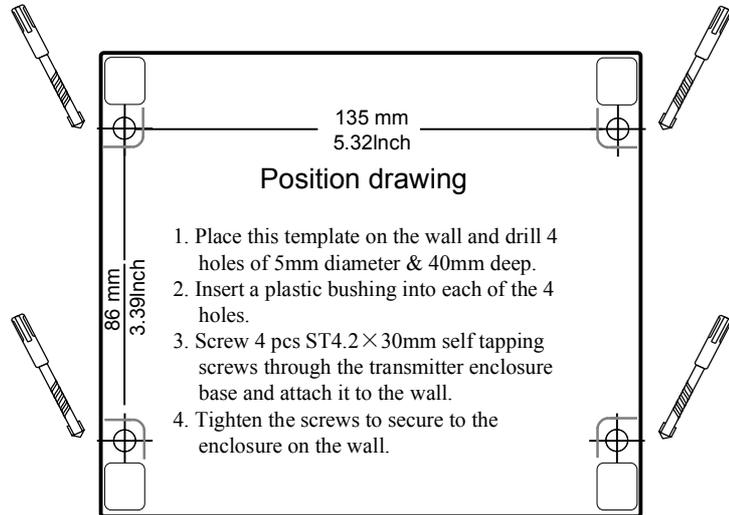
Take out the enclosed screws and plastic bushings. Insert the plastic bushings into the installing holes. Brackets will be installed at the bottom of the flowmeter. Put the flowmeter to the position and screw it in.
